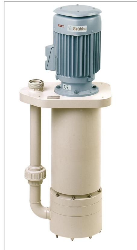
Depending on the operating parameters, either polypropylene (PP) or polyvinylidene fluoride (PVDF) is used for the production of the pump components. The series includes the types ETMB 25-125 and ETMB 32-125. Delivery capacity is up to 25 m<sup>3</sup>/h with head heights of 28 m at 0.37 to 3.0 kW drive ratings. Rotation speed range: 1450/2900 rpm or 50/60 Hz.
