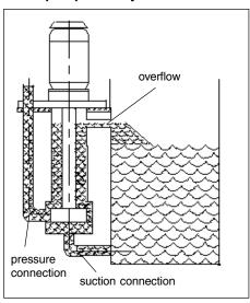
For the dry-well installation, the pump is arranged outside of the container.
