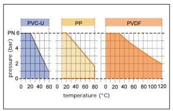
The pressure/temperature limits are applicable for the stated nominal pressures and a computed operating life factor of 25 years.
