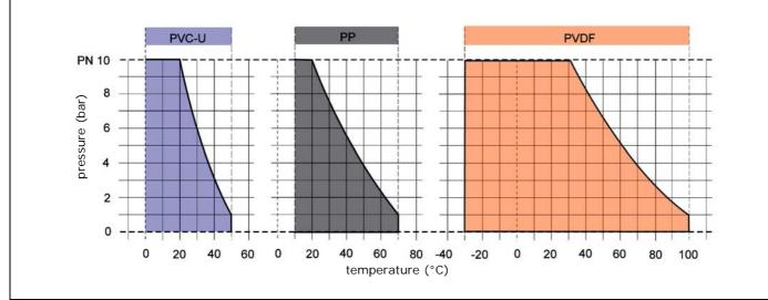
The pressure/temperature limits are applicable for the stated nominal pressures and a computed operating life factor of 25 years.
